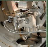
The function of the Double Crystal Monochromator (DCM) is to select and transmit X-ray radiation of the desired photon energy from an incident white synchrotron radiation beam.
