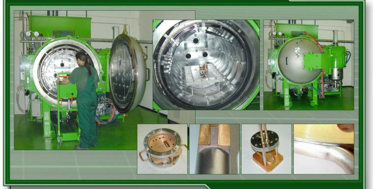
Since 2002 the company FMB GmbH has been working with its own High-Vacuum Heat Treatment Furnace.
